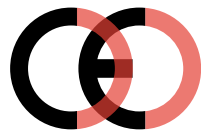
False CE Mark (too close)
